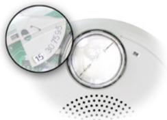
Genesis output levels are changed by simply opening the device and sliding the selectors to the desired settings. Settings remain visible through small windows on the device even after the cover is closed.
